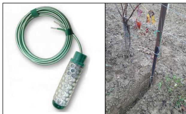
Figure 1 : Installation des sondes Watermark
